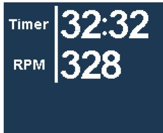
If you wish to use the device just as an orbital shaker and other modes are not needed, you can enable the simplified menu by holding the “PROGRAM” key and switching the network switch off and on again.
