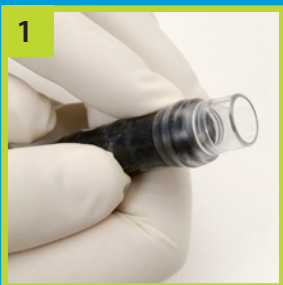
Attach Friction Fit Adapter Carefully twist or rock adaptor while pushing it onto distal end of scope.
