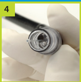
Secure Trip Wire Snap trip wire into first groove of inner cylinder.
