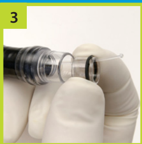
Position Inner Cylinder Position inner cylinder onto trip wire with edge closest to "O" ring facing outward.
