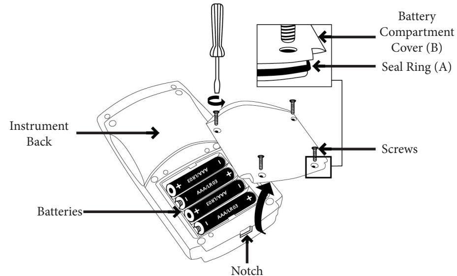
*To ensure that the instrument is waterproof:*
