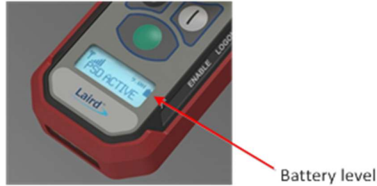
Figure 5: Battery Level Monitoring
