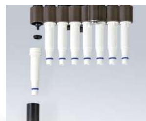
Individually exchangeable shafts on the Transferpette® S -8 and -12
