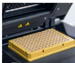
Thin-walled wells for reduced cycle times
