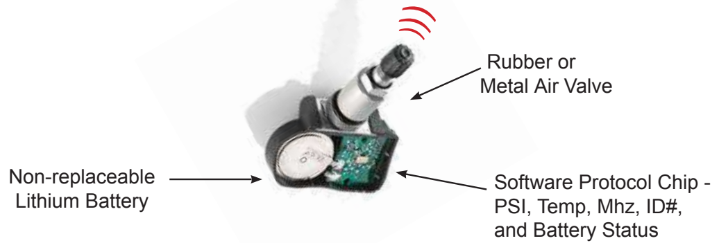
Tire Pressure Sensor Components
